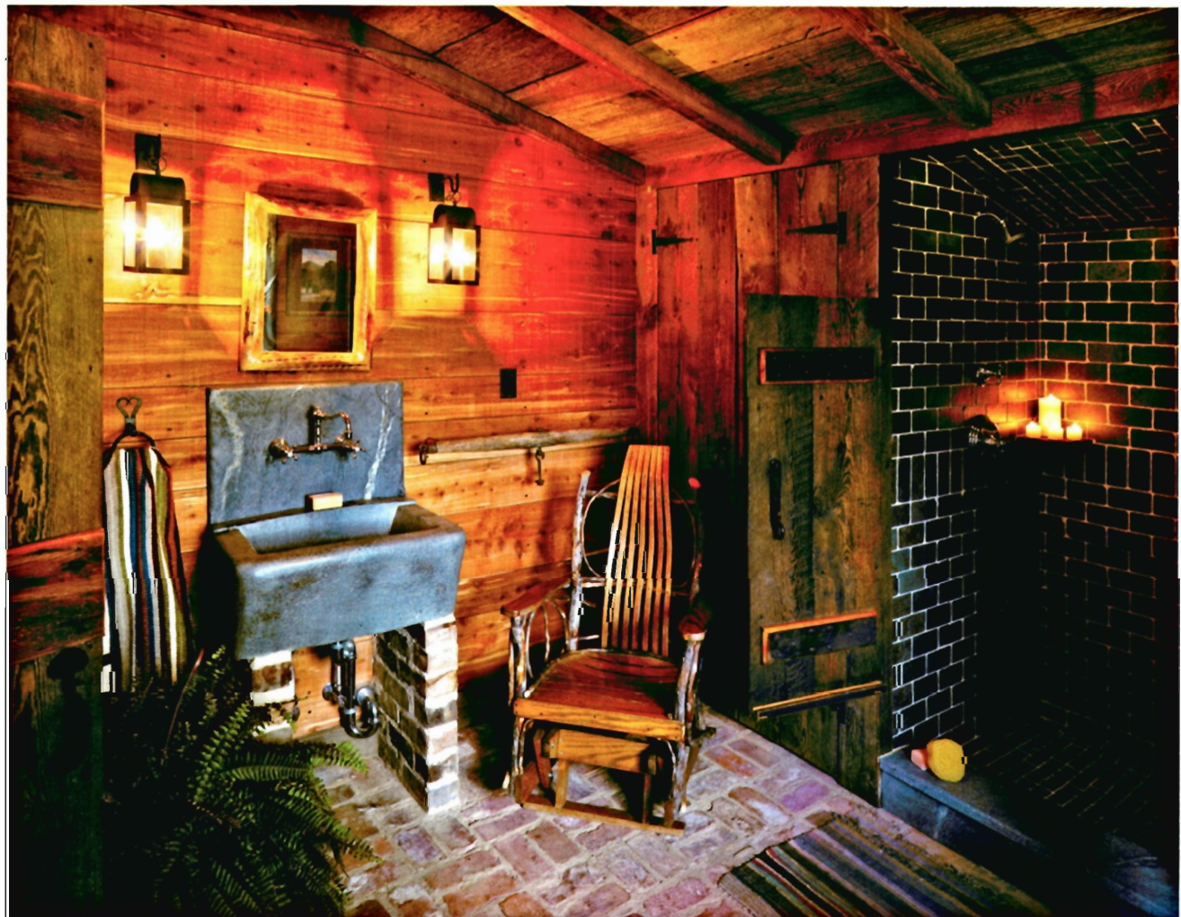
The sturdy sink, carved from a block of soapstone by Daniel Strumlauf, is one of many unique features in this room. The walls are eastern red cedar, which is native to the area while the barn-like doors that house the shower are regional yellow pine. The scent from the cedar enhances the relaxing mood of this room.
